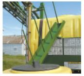
Stand consists of a 25-in. long, V-shaped trough fitted with four evenly spaced rods.
