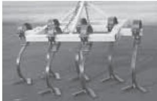
High-clearance shanks on cultivator leave room for debris to flow through.
