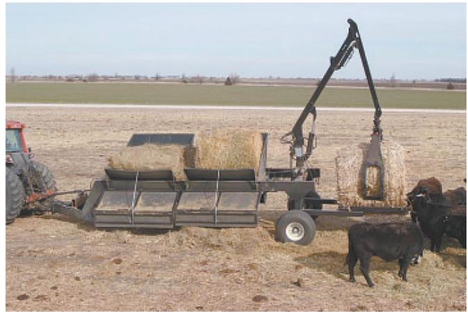
If bale plugs up in processor, grapple can be used to reposition it.
