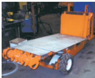
Front-powered rotor grabs bale to pull it up and onto cart platform.
