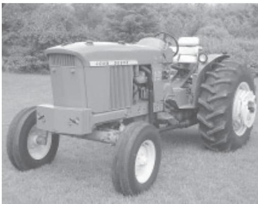
Robert Glanville is the owner of this 1964 Deere 3020 "utility tractor". The low profile tractor is built like an orchard tractor, but without the wheel flarings on back
