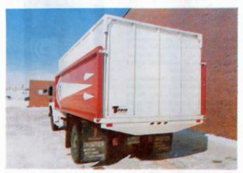
Metal silage liner is self-standing when not in use. It's expandable in width and length to fit virtually all truck boxes. Driver loads or unloads it alone in matter of minutes.
