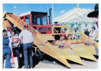
Vermeer offers four and six-row tractor-mounted corn pickers equipped with both sheller and husking bed attachments. A special frame mounts corn head onto front of tractor. The 3 pt. hitch carries either shelling or husking bed. Both units contain stands to make mounting and dismounting easy.
