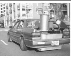
Wood gas generator turns wood and other biomass into gas to fuel cars, trucks, stoves and furnaces. Car shown above is running on syngas. A completely assembled unit is shown at right.
