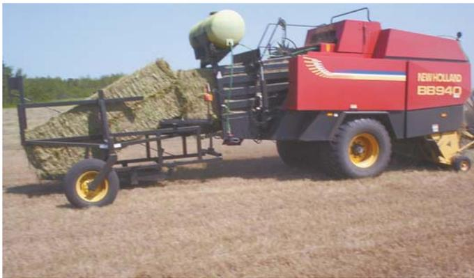
Caster wheel-mounted bale stacker is designed to always trail in line with baler's bale chute.
