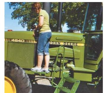
Non-slip fuel and access steps make it safer to work around Deere 20, 30, 40, 50, and 60 series tractors.
