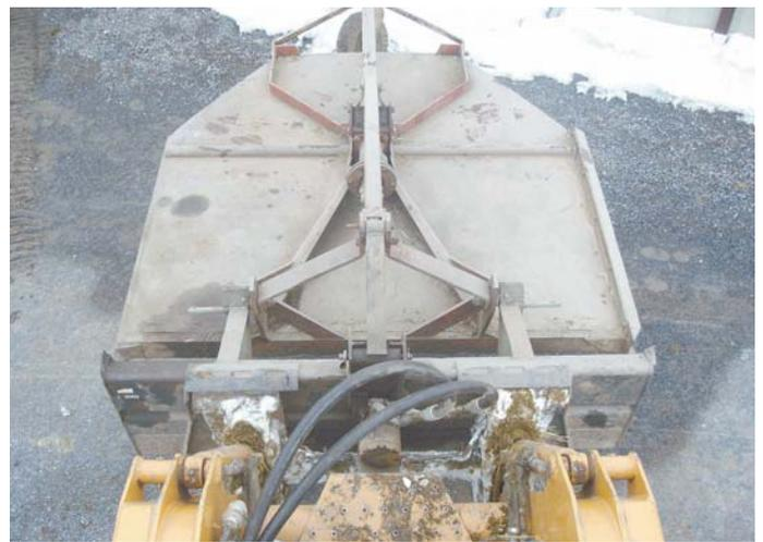
"I like the visibility and flexibility it gives me in thick brush," says Shirk, who turned a zero-turn rough-cut mower into a big mower by mounting it on skid steer loader arms.
