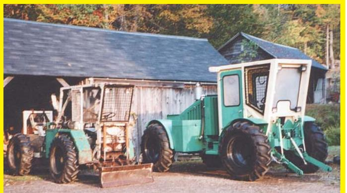
Back in 1991 FARM SHOW published a story on my front-mount 4-WD articulated tractor, which positions the operator right up front for perfect visibility. I still have the tractor, which is powered by a Ford 140 cu. in. 4-cyl. water-cooled gas engine, with both driver and engine protected by a wire brush cage. The 58 hp tractor is equipped with front or rear pto, front and rear 3-pt. hitch, foot-controlled hydrostatic 4-WD, center articulation and oscillation, and four 11.2 by 24 ag tread tires.
