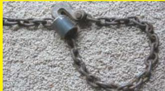
my "sure grip chain". It works to pull any size post. It consists of a length of chain, 2 hooks and a 1 1/4-in. pipe coupling. The hook that wraps around the post hooks to the short piece of pipe so it slides down the chain to tighten around anything. Works great and doesn't slip. **(Larry Zenz, Parks, Ark.)**
