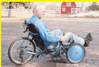
The rider sits facing forward with feet on the pedals up front, which chain-drive the rear wheel. The handlebars are used to lean the vehicle left or right. To shift gears, the rider uses twist grips on the upper ends of the handlebars.
