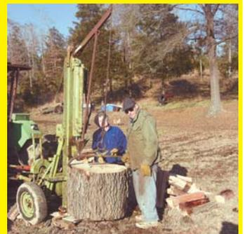
My home-built log splitter has a lift arm attached to the top. A 2-point grab hook lifts wood up to be split. The hook releases as the wood drops onto the splitter. The splitter can handle wood pieces that weigh up to 300 lbs. and measure 24 in. in diameter. **(Larry Zenz, HC 60, Box 154, Parks, Ark. 72950; ph 479 577-2677; zie7@ipa.net)**
