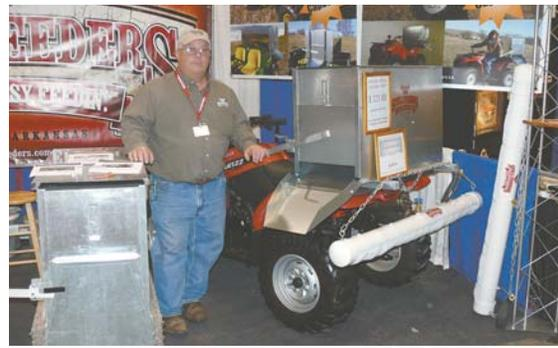
Randy Stull's gravity-fed feeder mounts on back of ATV.
