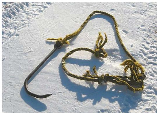
Designed to unplug round balers, hay hook is made from sucker rod bent into the shape of a giant fish hook.
