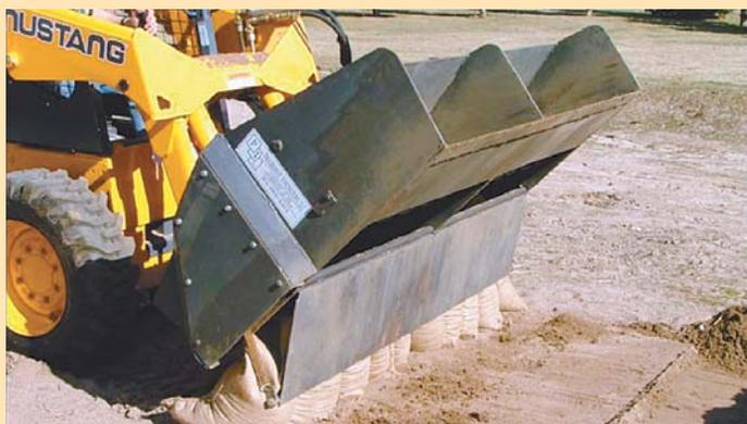
Sandbagger attached to skid loader is designed to fill 12 bags at a time. It's basically a large scoop with 12 sets of bag holders on back.
