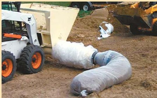
Instee Levee Builder lays an 18-in. high barrier 400 ft. long in less than an hour. An auger delivers material out the side to a 6-mil poly sock.
