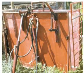
He added a 2-way valve and a hydraulic cylinder, which are powered by a small tractor.
