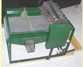
When the treadle is pumped up and down, connecting rods turn the reel and shake the screen.
