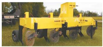
$\bf A$  16-in. coulter precuts sod layers, and is followed by a shank and coil spring-mounted packer wheel.
