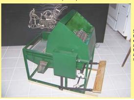
Small-scale thresher consists of a foot treadle, an enclosed threshing reel, and a winnowing
