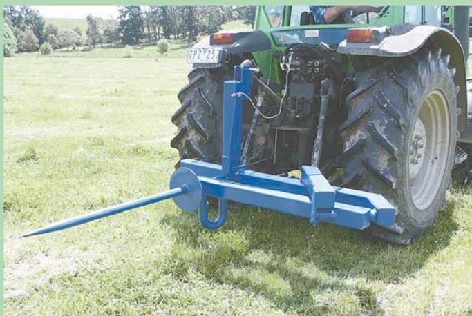
Bale handler's frame is designed with a spike that holds bale at an angle.
