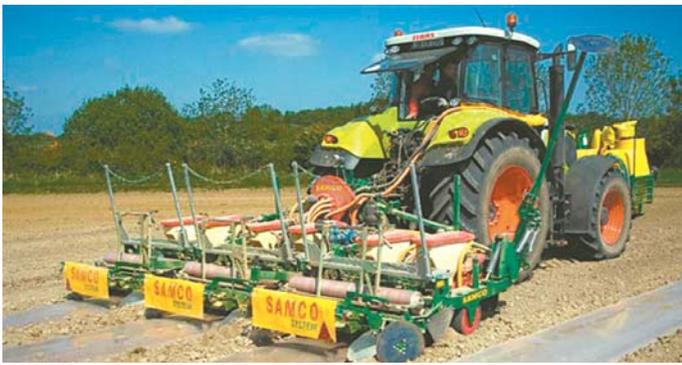
Developed in Ireland, the Samco planting system applies herbicide and plants the corn under 55-in. swaths of specially designed, degradable plastic.
