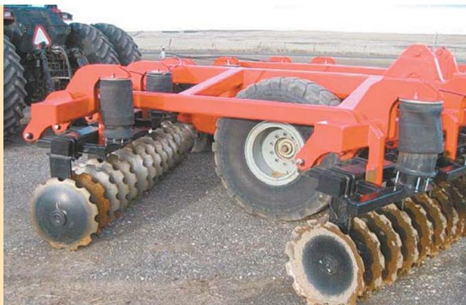
Disk's large truck tires provide extra flotation and minimize tire tracks.
