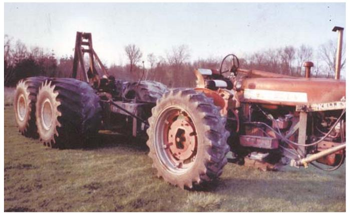
Deane and Dan Sarber built two different "winches on wheels" to pull out stuck machines. Model shown above rides on four big flotation tires off a Big A self-propelled sprayer.
