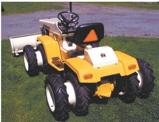
The tractor still has the original dash, seat, and gearshift lever from the 1450. Naragon added an aftermarket muffler designed for a Ford 8N tractor that's equipped with a stainless steel stack.
