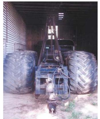
Self-propelled, 4-WD tandem axle winch is designed to lift stuck machine straight up and then pull it out. Cable rides up and over winch on tower at back of machine.
