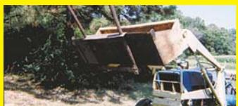
on my Ford 4000 tractor. The 6-ft. long spears are spaced 32 in. apart and welded through holes in a heavy angle iron bracket that slips over the lip of the bucket. The spears extend through the angle iron and under the bucket, and are
