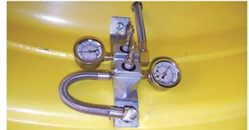
Tire Minders fit single, dual and triple wheels. Photo shows a 2-gauge unit for duals.
