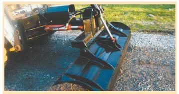
Jason Tobin designed this skid loader-mounted blade for pushing, dragging, cutting and leveling work. "The blade can be tilted and rotated to any angle you want," he says.
