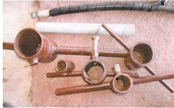
Cutter bolts screw into a variety of sizes of copper pipes which are used to slice plastic pipe into spirals that slip over hydraulic hoses to protect them.
