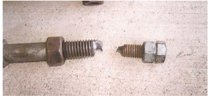
Cutters are made by fashioning points onto ends of bolts.
