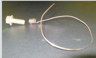
**Roger Gutschmidt, Gackle, N. Dak.:** He uses a simple trick to get bolts through openings where you can't get your fingers inside. He wraps a piece of .035 welding wire tightly around a 5/16-in. bolt.
