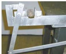
Original machine had just one position for the jaws, while the redesigned version comes with two positions.
