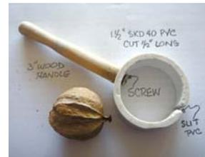
Nut fits inside 1 1/2-in. dia. pvc pipe screwed to 3-in. long wooden handle. Slit in pipe allows pipe to expand as nut is smashed.
