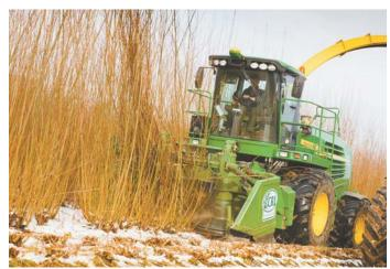
$Hy draulically-driven\ willow\ header\ fits\ a\ wide\ range\ of\ forage\ harvesters.\ It\ can\ harvest\ up\ to\ 150\ tons\ per\ day\ of\ chipped\ wood.$
