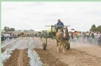
One-horse, high-clearance sprayer has an 85-gal. tank and two 10-ft. manual lift booms.
