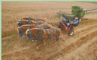
A 74 hp diesel pto forecart mounted on cart behind horses powers combine.
