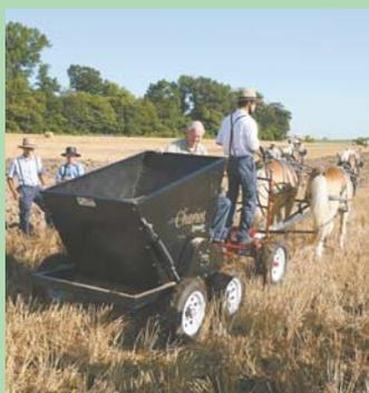
Horse-pulled, 30-bu. manure spreader can be powered by a ground-drive unit or hydraulic drive.
