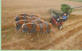
A 74 hp diesel pto forecart mounted on cart behind horses powers combine.
