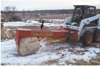
Log splitter is built from two pieces of channel iron mounted back to back, with an 8 by 24-in. "window" in between.
