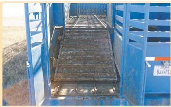
Trailer has a 10-ft. long compartment at front, followed by two 15-ft. compartments – each with its own gate.
