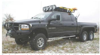
Doug Loughery stretched, raised and rebuilt his 2006 Dodge 3500 pickup to end up with this 27-ft. long, 6-WD "Mega Cab" truck.
