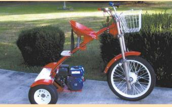
Tricycle rides on a 21-in. high front wheel off a motocross bike and two 8-in. boat trailer rear wheels, which are chain-driven off the engine.
