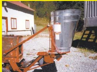
a Herd 3-pt. hitch mounted broadcaster to the front of a Gravely garden tractor. We used a Boston gear #621A speed reducer to get the proper drive shaft direction and speed off the front pto. The seed gate is foot-operated for quick start and stop when broadcasting.
