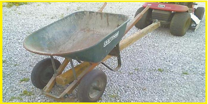
I found an easy way to turn a wheelbarrow into a cart I can tow behind a garden tractor or ATV. I bought an 8-ft. 4 by 4 and laid it over the axle between the front wheels. A couple brackets wrap around the axle and lag-bolt to the 4 by 4 to hold it in place. The wheelbarrow is stock, except for the brackets. A bracket attached to the opposite end pins to the drawbar hitch.
