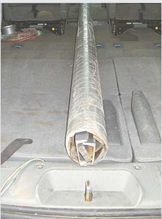
**Roger Gutschmidt, Gackle, N. Dak.:** "Here's a tip that allows you to comfortably haul quite a few 10-ft. lengths of steel in your mini van without getting the interior dirty. For the last 10 years, I've been using a 5-in. dia. cardboard tube that once held a roll of new carpet. Instead of discarding it, I wrapped the tube with duct tape so it can be wiped off if it becomes dirty, and position it down the center of the van whenever I go to town to buy steel.
