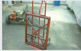
a length of flat steel serving as a brace at the bottom. The brace is what the front rides on during transport.
