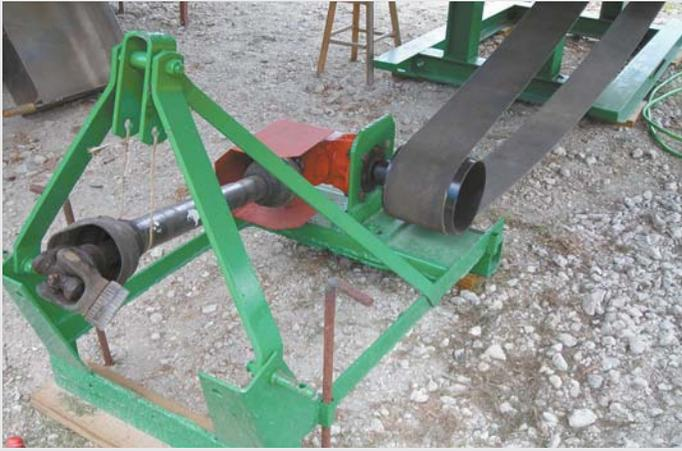
**Lonnie Fisher, Baytown, Texas:** "I needed a flat belt drive system to operate my Chattanooga 44 cane mill, but none of my tractors had a flat belt pulley. So I turned the gearbox 90 degrees on an old Rhino 5-ft. mower and
