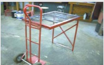
**Eric McNutt, Sulphur Springs, Ohio:** "My home-built welding table makes use of a simple 2-wheeled dolly and folds up for transport and storage. As a result, the table doesn't take up much more storage room than the dolly itself.
