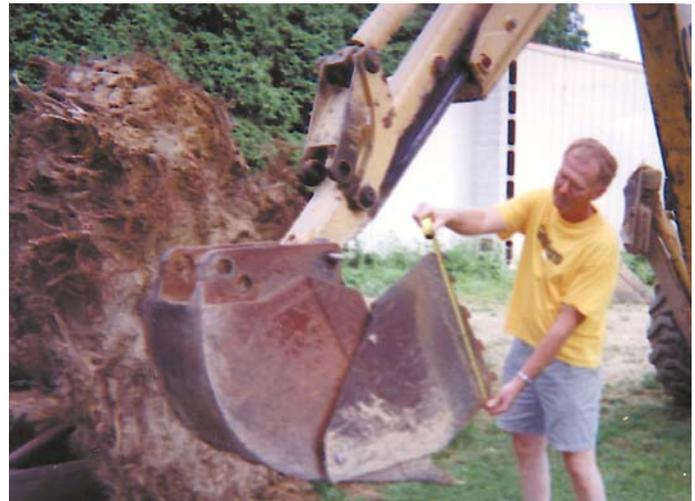
Toothed cutter plates extend beyond joint of backhoe arm and bucket, allowing Conn to saw through frozen ground.
