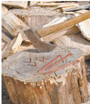
Three 6 to 7-in. "spikes" stick up from top of wood block to hold chunks in place for splitting.
