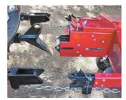
As a fifth wheel support system (left), hitch duplicates the standard front axle on a 34 or 1-ton truck. Unit attaches to truck at 3 points with locking pins (right).
