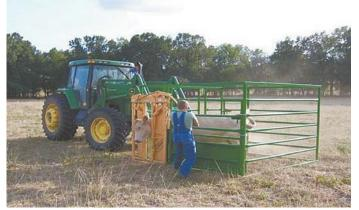
"Mobile Clinic" attaches to front-end loader. If necessary, animal can be transported on a floor section that drops down by headgate
