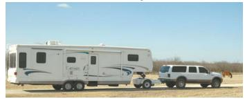
Automated Safety Hitch acts as a drop axle, turning a single axle towing vehicle into something "better than a dually".
