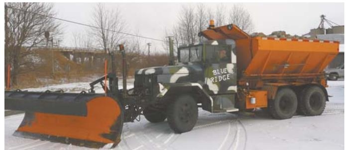
Chris Kirkland converted a 2 1/2-ton Army truck into this snowplow/salt truck. It has an 11-ft. wide blade on front and a live floor box on back.
