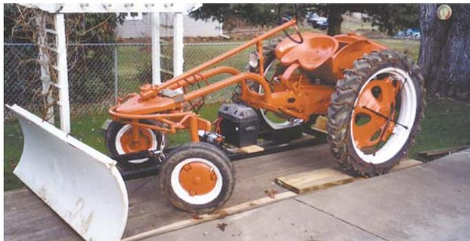
Ivan Pettit designed a snowplow to fit his 1949 Allis Chalmers G tractor. It’s raised and lowered by an electric winch.
