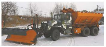
Chris Kirkland converted a 2 1/2-ton Army truck into this snowplow/salt truck. It has an 11-ft. wide blade on front and a live floor box on back.
