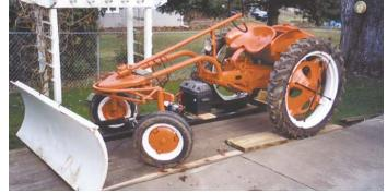
Ivan Pettit designed a snowplow to fit his 1949 Allis Chalmers G tractor. It's raised and lowered by an electric winch.
