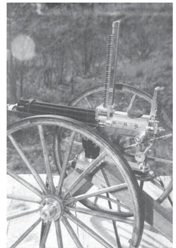
Half-size 1800's-style Gatling gun uses 50-round clips of .22-caliber ammunition, fired by a battery of 10 rotating barrels.
