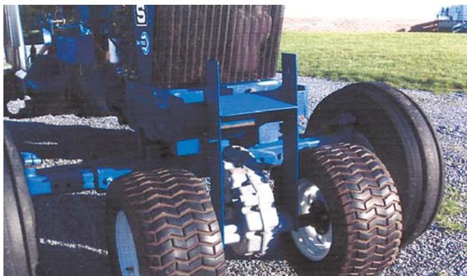
Front-mount bale unroller uses the rear axle and wheels off an old riding mower. The 16-in. wheels spin freely. Weaver simply drives forward, pushing wheels against bale.
