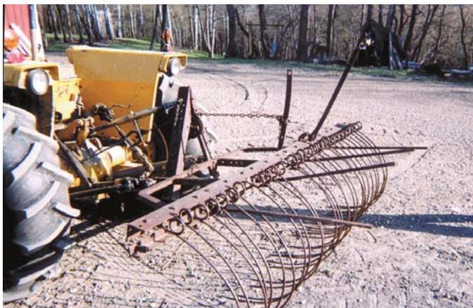
**Gabe Davidson removed the wheels and seat from an old horse-drawn rake, then made brackets to mount it on a tractor 3-pt.**
