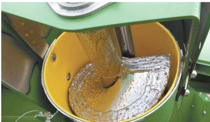
**Poly tank fill tube liner bolts on inside the original fill tube.**
