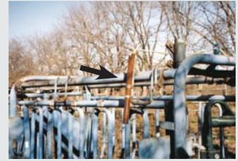
Photos show pipe handle added to chute to make it easier to use.
