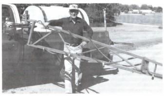
My mid-mounted pickup sprayer subjects the booms to less than one half the movement and road shock of a conventional rearmounted pickup sprayer. The booms on the sprayer mount on angle iron brackets just behind the cab. In transport they're held in alongside the pickup box. In the field they're allowed to swing freely to their extended
