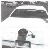
This magnetic backup mirror sticks to the back of a car trunk or pickup tailgate to make hitch-ups easier. It has a strong magnetic
