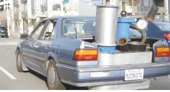
Wood gas generator turns wood and other biomass into gas to fuel cars, trucks, stoves and furnaces. Car shown above is running on syngas. A completely assembled unit is shown at right.
