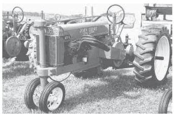
Bruce Bauer put a Chevy 350 V-8 engine into a 1938 Deere Model A tractor.
