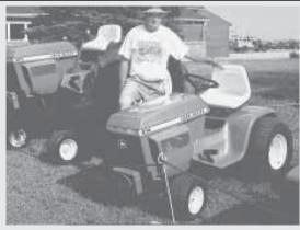
Prom replaced the original 14 hp engine on his Deere 214 garden tractor with a 50 hp Chevy Geo Metro 3-cyl. engine. Tractor still has its original ventilated side covers.
