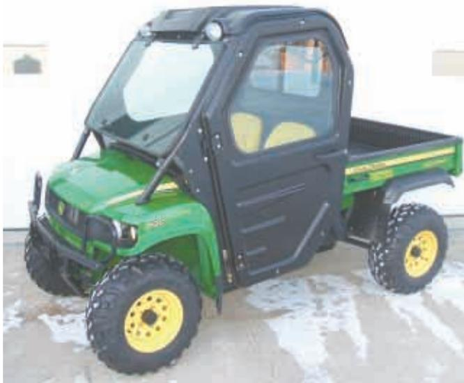
Cab bolts onto Gator's standard rollover protective structure. Cab's roof and doors are made from heavy-duty ABS plastic and mount on a steel frame.
