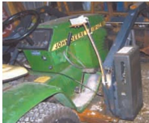
**Electric-operated wheelchair lift - designed for a school van - was converted into a quick-tach front-end loader. Inventor Tom Chaney uses it on his Deere garden tractor.**
