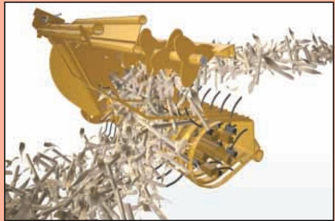
**Power-driven rotor helps feed bulky crop residue into baler with minimal plugging.**
