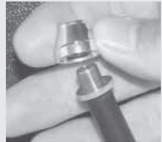
**Snap-on magnetic valve stem cover replaces “screw-on” dust caps.**
