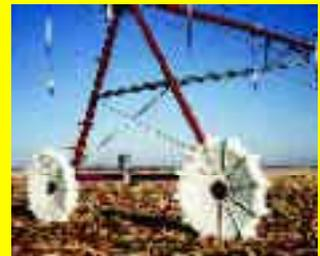
have a tractor tire lug design that fills up with mud, causing the wheel to spin and get stuck. The cleats on our wheel are deep and are spaced farther apart. Also, they go straight across both sides of the wheel like the lugs found on old-time tractors with steel wheels. The result is that they're far less likely to get stuck.
