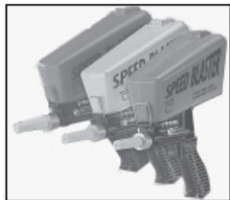
a replaceable ceramic nozzle, and is quick and easy to use. Just pour in some sand, plug in the air compressor, put on eye protection, and step outside. The design uses gravity to help force the blast media into a hardened steel mixing chamber. Compressed air then forces the particles through the ceramic nozzle at high velocity. It works great every time, and it's American-made."
