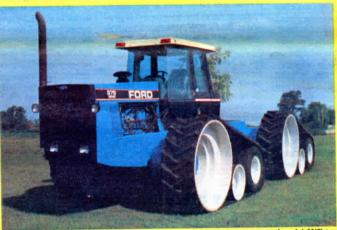
Kelderman's conversion system turns a conventional 4-WD tractor into an extremely maneuverable 4-tracked tractor that exerts even less pressure per square inch than Caterpillar's rubbertracked Challenger tractor, virtually eliminating compaction.
