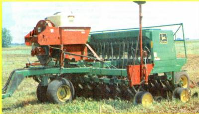
To plant corn with his Deere 750 drill, Beckman equipped it with an International air planter. Seed tubes run from the Cyclo hopper to 6 row units. He injects dry starter fertilizer using row units on either side of the row of corn, carrying fertilizer in the drill's seed hopper.
