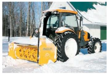
Snowblower is equipped with shield that rotates 180 degrees to cover either front or back of aug er. Operator here is blowing snow while moving backward.
