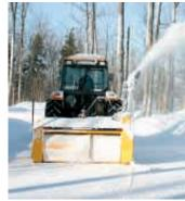
By rotating shield to cover back of auger, operator can blow snow while driving forward.
