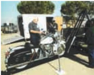
One-man motorcycle loader attaches to bed of pickup and can also be mounted on a trailer. It consists of a frame with an electrical-powered mounting rail in it.
