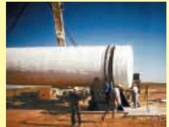
Manure from hog barn is continuously composted in drum-type composting rig.
