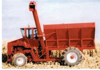
Bob Wright built this self-propelled grain cart using the wheels, axle and engine off an old International combine. It's fitted with a 400-bu. tank.
