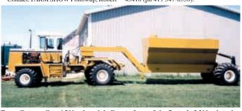
Terra-Gator pulls a 4,200-gal. tank built out of one of the floater's 3,200-gal. tanks. Note a pplication toolbar on back. Unit can go down the road at 40 mph.
