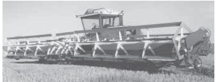
Moellenbeck says his swather is 14 ft. wider than the largest commercial swather. It's powered by a Caterpillar 3145 diesel and folds up for transport (below).
